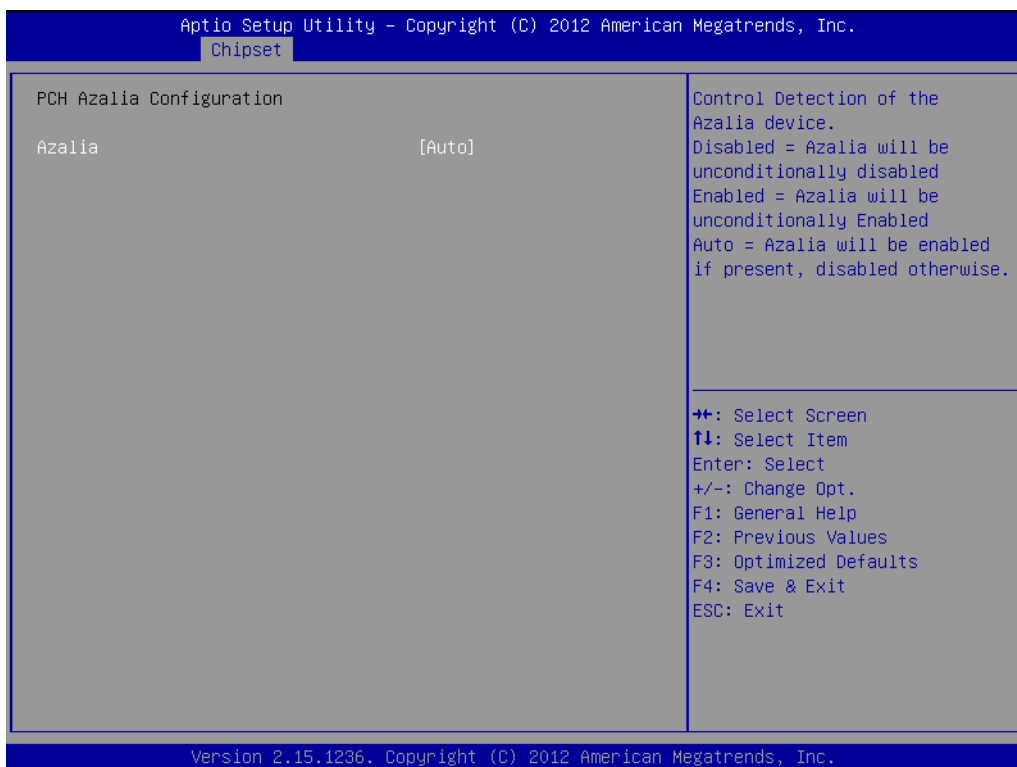
Figure 3.26 PCH Azalia Configuration
