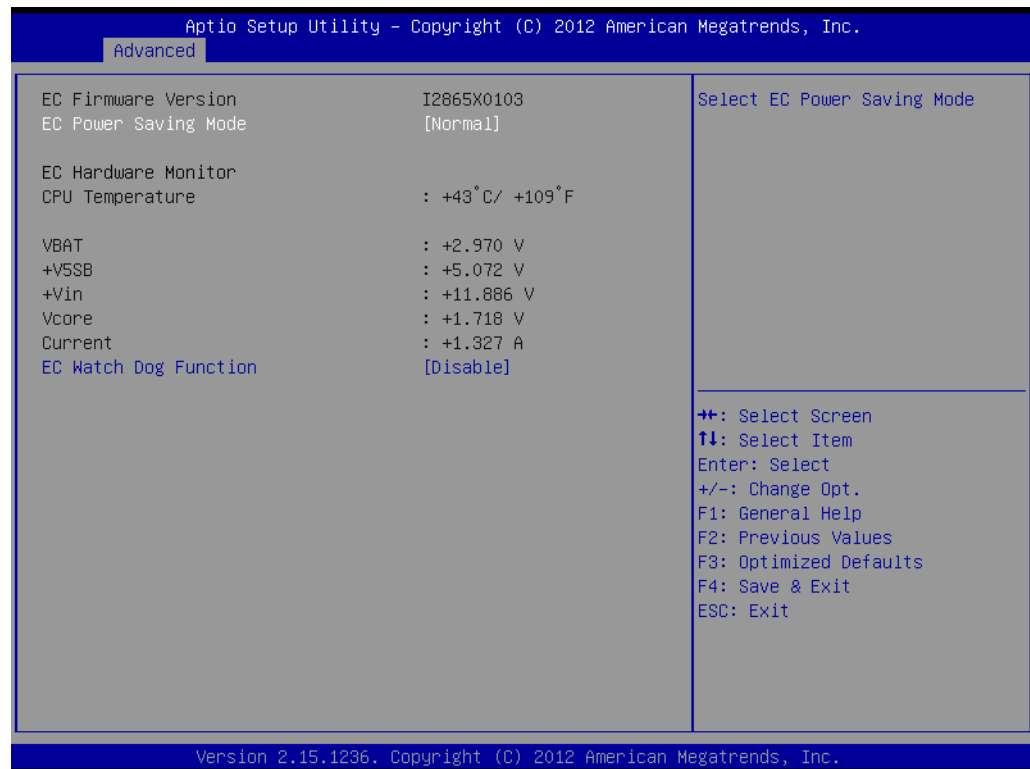
Figure 5.15 Embedded Controller Configuration
