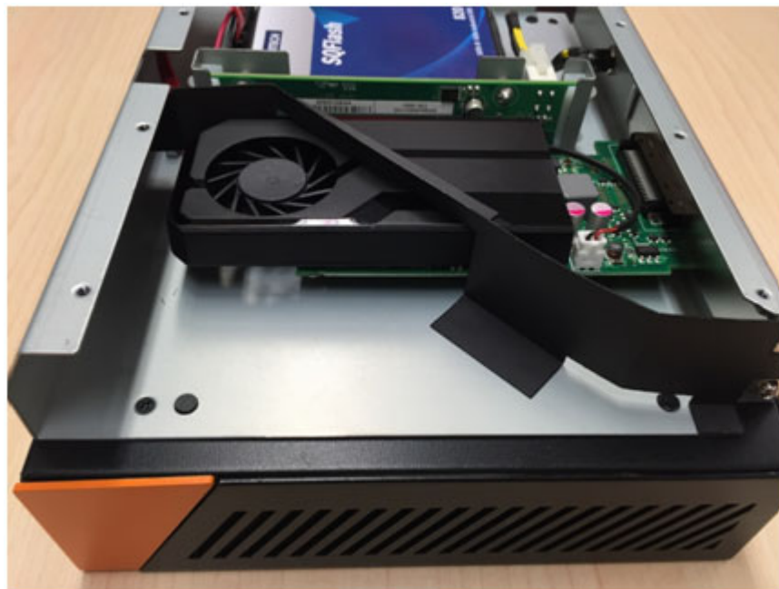
Figure 3.7 Fan duct location (2)
