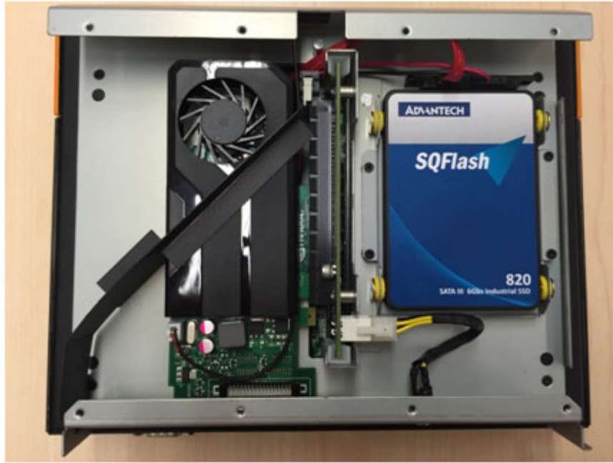
Figure 3.6 Fan duct location (1)
