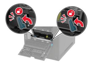
**3** Remove the used fuser.
