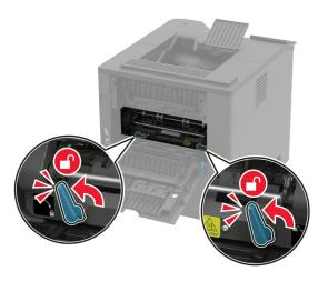
Remove the used hot roll fuser.
