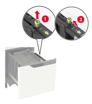
**b** If the A5 length guide is still attached, then remove it. If the guide is not attached, then proceed to <u>step</u> <u>d on page 33</u>.
