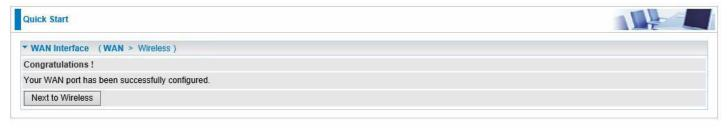
**5.** After the configuration is successful, click **Next to Wireless** button and you may proceed to configure the Wireless setting. The device supports dual-band wireless connections, in Quick Start part, users can only enable or disable the wireless on the band and the exact SSID and encryption Key (1. Leave it empty to disable the wireless security; 2. Fill in the Key, and the encryption mode will be WPA2-PSK/AES). For detail setting, please go to the Wireless part in this Manual.
