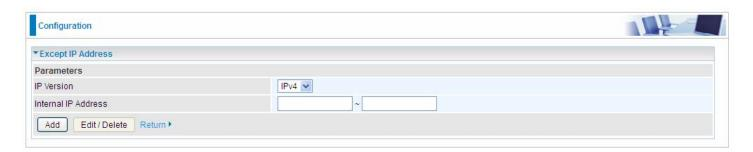
Enter the except IP address. Click **Add** to save your changes. The IP address will be entered into the *Exception List*, and excluded from the URL filtering rules in effect. For specific process, please refer to *Keywords Filtering*.
