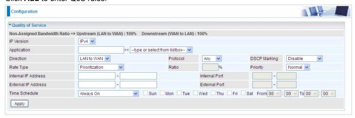
IP Version: Select either IPv4 or IPv6 base on need.
