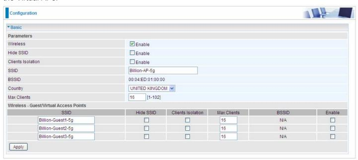
Wireless: Default setting is set to Enable. If you do not have any wireless devices, check the checkbox again to unselect.
