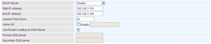
**Start IP Address:** The start IP address of the range the DHCP Server used to assign to the Clients.
