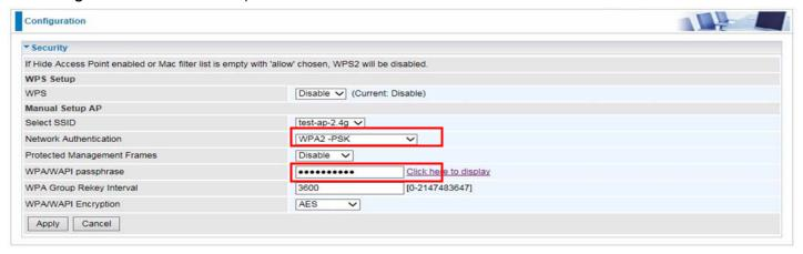
III. Advanced wireless configuration for Router A (Channel 1, Bandwidth 20MHz/40MHz, OBSS Coexistence Disable). Note: Select your own bandwidth, but both sides need to be same.
