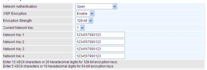
**WEP Encryption:** Select to enable WEP Encryption.
