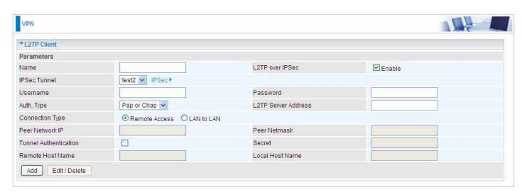
IPSec Tunnel: Select the appropriate IPSec for L2TP rule configured for the L2TP Client.
