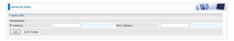
**IP Address:** Enter the IP of the device that the corresponding MAC address will be mapped to. **MAC Address:** Enter the MAC address that corresponds to the IP address of the device.
