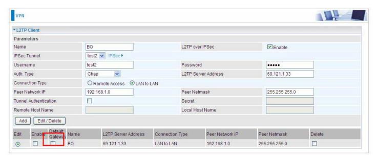
**Note:** users can see the "Default Gateway" item in the bar, and user can check to select the tunnel as the default gateway (default route) for traffic. If selected, all outgoing traffic will be forwarded to this tunnel and routed to the next hop.
