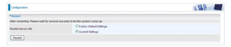
If you wish to restart the router using the factory default settings (for example, after a firmware upgrade or if you have saved an incorrect configuration), select Factory Default Settings to reset to factory default settings. Or you just want to restart after the current setting, the select the Current Settings, and Click Restart.
