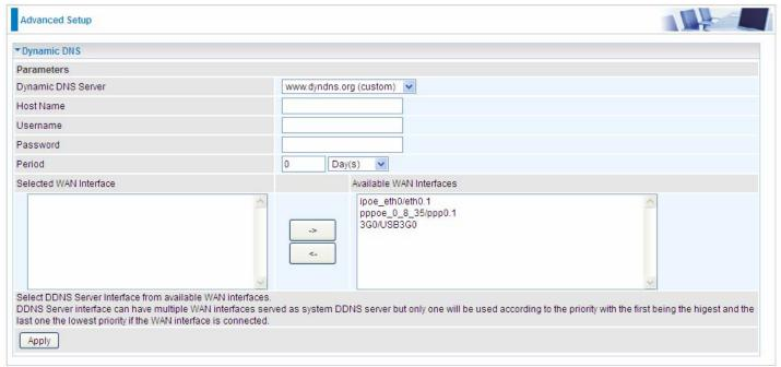
You will first need to register and establish an account with the Dynamic DNS provider using their website, for example <a href="http://www.dyndns.org/">http://www.dyndns.org/</a>
