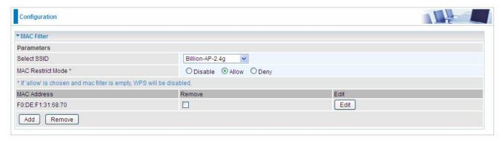
To delete entries, check the remove checkbox and press **Remove** to delete it.
