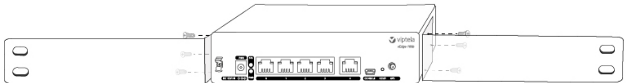
Figure 2: Attaching the Mounting Ears to the vEdge 100b Router Chassis
