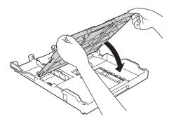
6. Load up to 20 sheets of photo paper with the printing surface **face down**. Loading more than 20 sheets of photo paper may cause paper jams.
