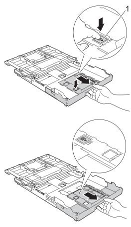
5. Gently press and slide the paper width guides (1) and the paper length guide (2) to fit the paper size.
