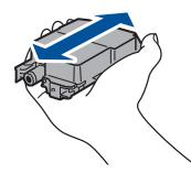
4. Insert the ink cartridge in the direction of the arrow on the label.
