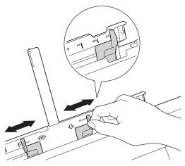
4. Load only one sheet of paper in the manual feed slot with the printing surface **face up**.
