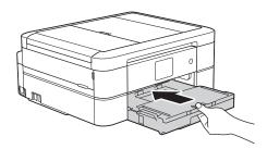
6. While holding the paper tray in the machine, pull out the paper support (1) until it locks into place, and then unfold the paper support flap (2).
