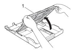
4. Gently press and slide the paper width guides (1) to fit the paper size, and then lift up the stopper (2).
