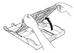
5. Wipe the inside and the outside of the paper tray with a dry, lint-free cloth to remove dust.
