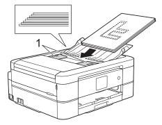
4. Place your document, **face down**, **top edge first** in the ADF underneath the paper guides until you feel the document touch the feed rollers and the LCD displays [ADF Ready.].
