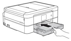
7. Pull out the paper support (1) until it locks into place, and then unfold the paper support flap (2).
