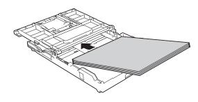
Make sure the paper is flat in the tray and the paper length guide (1) touches the edges of the paper.
