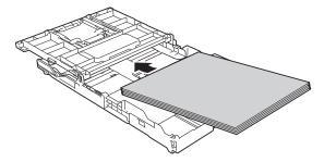
Make sure the paper is flat in the tray and the paper length guide (1) touches the edges of the paper.
