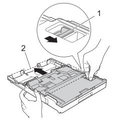
4. Load up to 20 sheets of Photo or Photo L paper in the photo paper tray with the printing surface **face down**. Loading more than 20 sheets of photo paper may cause paper jams.
