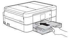
10. Pull out the paper support (1) until it locks into place, and then unfold the paper support flap (2).
