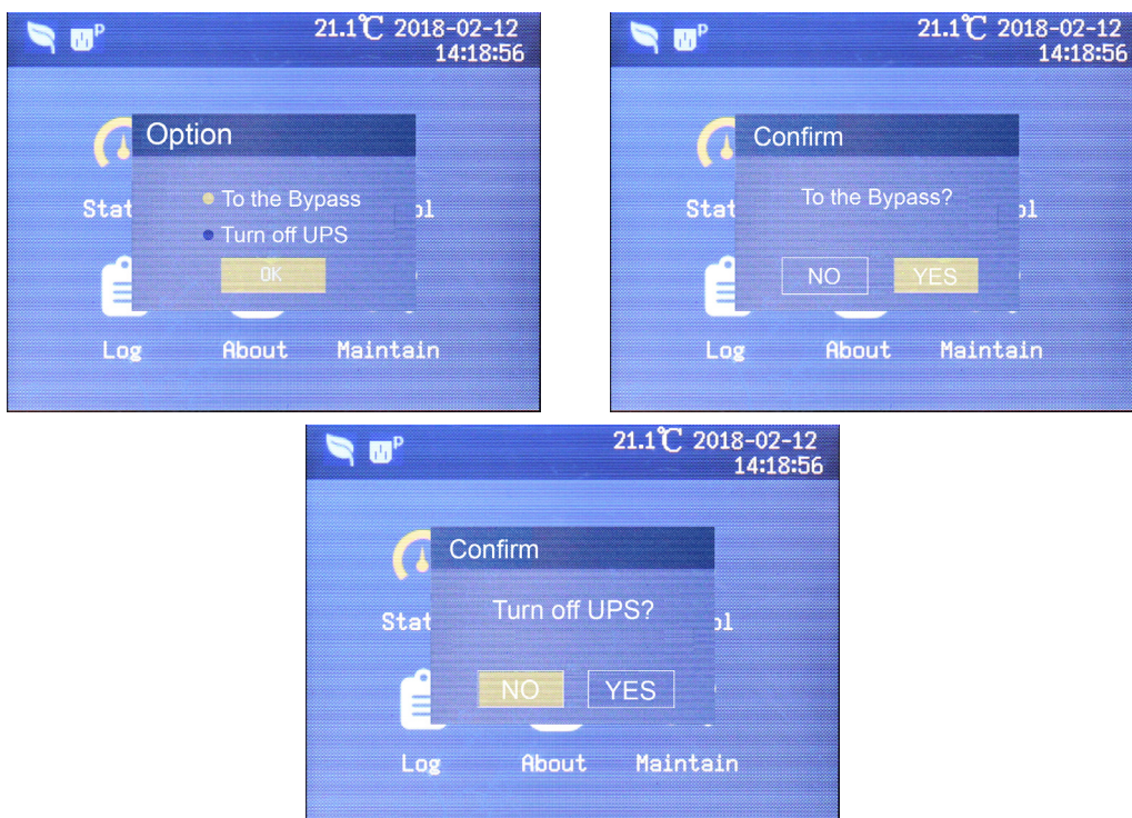
Figure 52 Bypass normal interface
