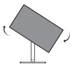
4 Complete the installation by rotating the monitor 90° as shown below.
