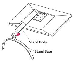
4 Turn the screw clockwise to secure the **stand base**.
