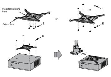
A Screw D Tightening torque: 8kgf-cm (≤12kgf-cm)
