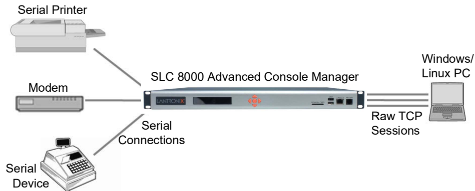
Figure 11-4 Multiport Device Server
