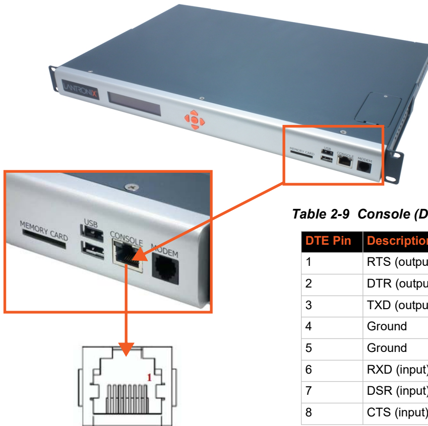
Figure 2-8 Console Port (Front Side)
