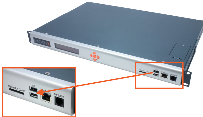
Figure 2-12 Dual USB Ports
