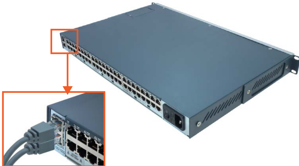
Figure 2-10 Dual Ethernet Network Connection
