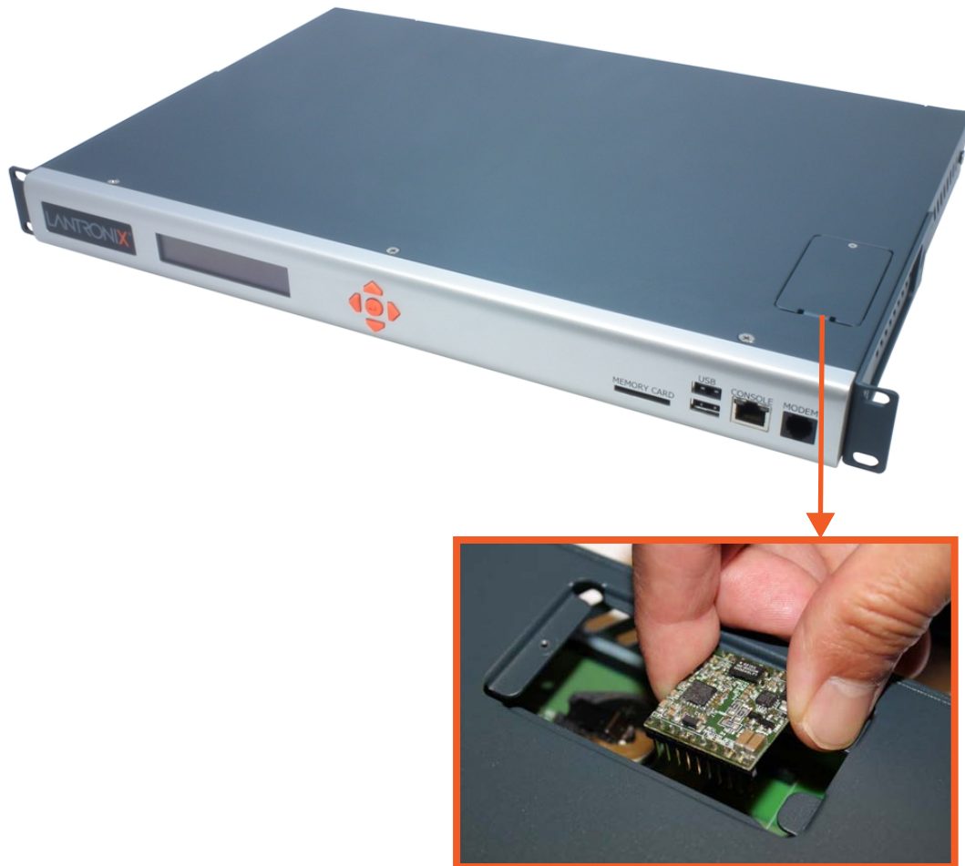
Figure 2-14 Internal Modem Location
