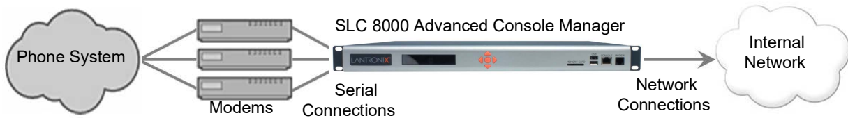
Figure 11-2 Remote Access Server
