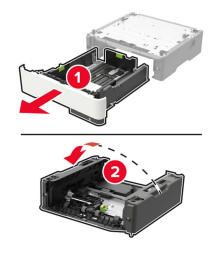
**5** Remove the used pick roller assembly.
