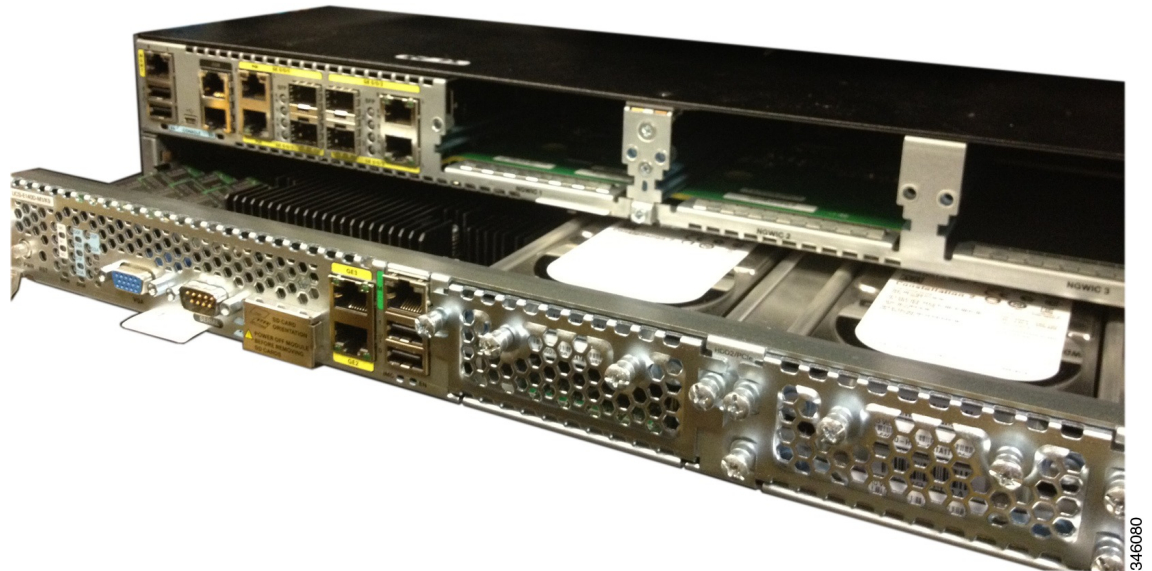
Figure 7: Double-Wide E-Series Server in a Cisco ISR 4000 series
