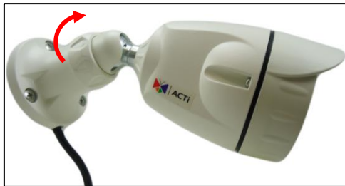
Sample of Wall Installation
