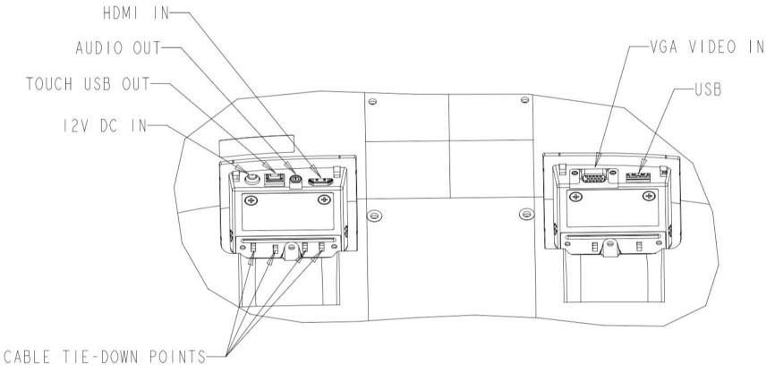
Note: Cable tie-down points can be used to tie down the cables with tie wraps. Simply loop the tie wraps through the cable tie-down points and around the cable to secure cable connections.
