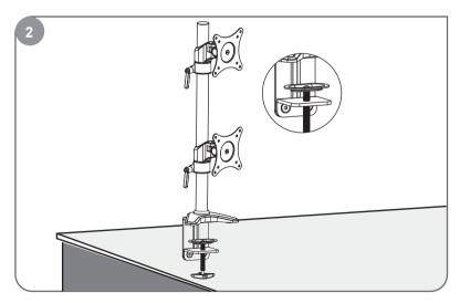
Tighten clamp using clamp screw until mount is securely fastened to desk.
