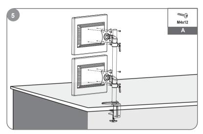
Flush surface installation: Install 4 screws through faceplate to monitor via mounting holes.
