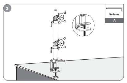
If space is still not enough for clamp,remove clamp screw and attachment entirely and reattach clamp screw with attachment upside-down.
