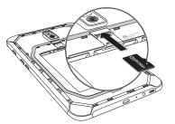
4. Insert the battery, making sure to align the gold contacts and press down.
