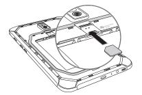
3. Slide the memory card into the card slot until it is secured.
