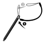
Insert the other loop end to the tether holder on the Tablet PC (as indicated by ① below). Then, insert the stylus end through the loop (as indicated by ② below) and pull it tight.
