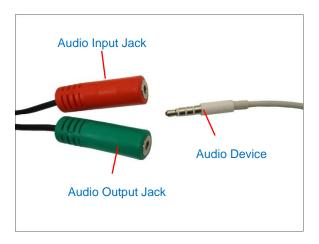
**NOTE 1:** Make sure that the connected audio input device has a built-in amplifier. Connecting an ordinary microphone will dwarf sounds and will result in inaudible recording.
