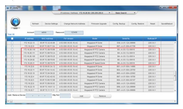
The camera model name is shown on the list. Click on the IP address to automatically launch the default browser of the PC with the IP address of the target camera already filled in the address bar of the browser.
