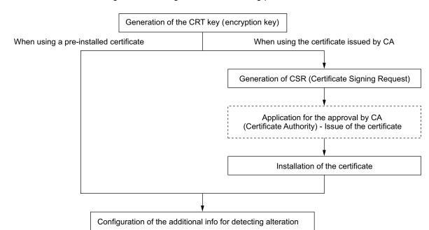
The alteration detection settings will be configured in the following procedure.
