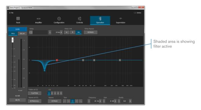
**5-band parametric equalizer (PEQ):** Filters can be edited by mouse, scroll wheel or entering parameter values. While editing via mouse and scroll wheel are instantaneously, editing numeric values (figures turn to orange) needs to be confirmed with "Enter".
