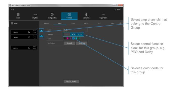
Example above is showing a group "Subs" with assigned channels A of the first two amplifiers. PEQ and Delay are selected as common control function blocks for all "Sub" channels.
