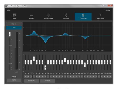
**31-band graphical equalizer (GEQ):** B allows bypass of an individual filter. Display resolution can be adjusted with right mouse click and scroll. Group level, mute and metering are available on the left side. Flatten puts all filters back to 0, double-clicking a fader will reset to the 0dB position, a bypass makes the GEQ inactive.
