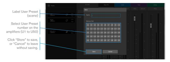
As soon as you select a User Preset number (U01 to U50) and click "Save", the current setting with the label in the display is saved in the project files while all the actual parameter settings are saved into all connected amplifiers and the project file.
