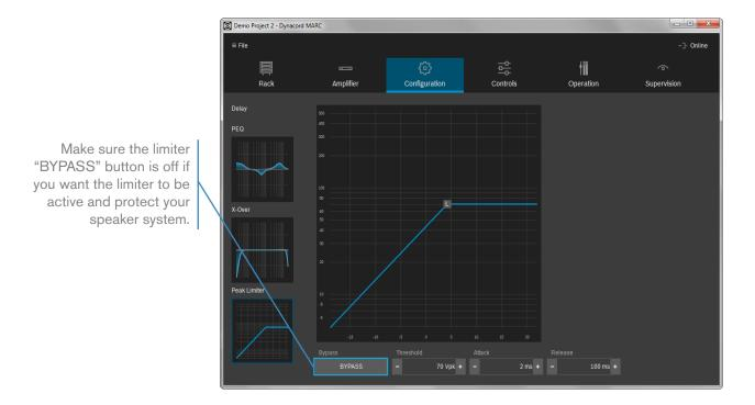
**Peak-Limiter:** You can enter values for threshold, attack and release. The limiter is only active if "Bypass" is deactivated.
