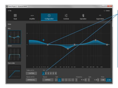
You can activate a filter by clicking and moving the number in the frequency curve, or in the EQ selector.
