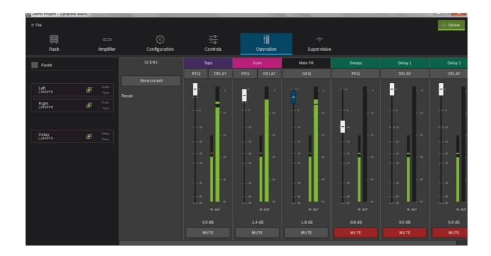
If you click on "Operation", you can now start controlling your amplifiers in real time. If signal is present, the VU metering will display input and output signals.
