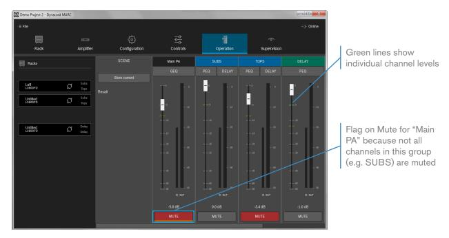
Mute or Unmute are always executed for amplifier channels assigned to the control group. If a channel is assigned to multiple groups, always the last action is followed. Depending on channel assignment this can cause an "error flag" on a mute button, indicating that some group members have been unmuted since the group mute was activated.
