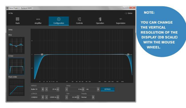
**X-Over Section:** Hi-Pass and Lo-Pass (Linkwitz-Riley 12dB, 24dB, Butterworth/Bessel 12dB, 18dB, 24dB, underdamped 12dB, 6dB slope) gain trim, polarity, alignment delay.
