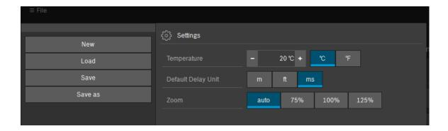
Settings will let you adjust temperature for delay calculation, default delay units and zoom factor (size) of the MARC program.
