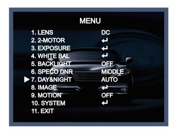
◆ AUTO : Automatically, It shifts into the color mode in the bright environment and the B/W mode in the low light condition. It can adjust the delay time, starting brightness and end brightness according to the ambient conditions by pressing the Set button.
