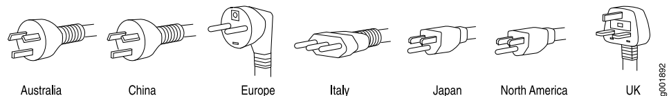
Figure 12: AC Plug Types
