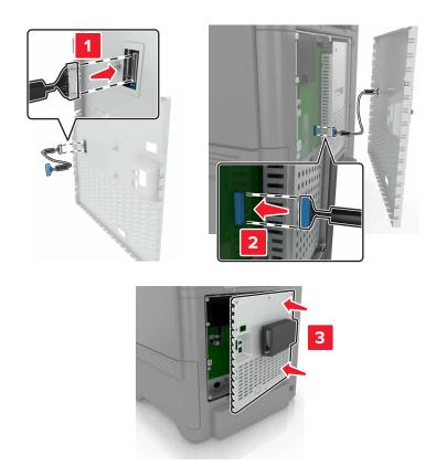
7 Reattach the controller board access cover.
