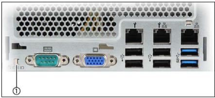
Figure 204: Indicators on the connector panel: CSS, Global Error and ID indicators
