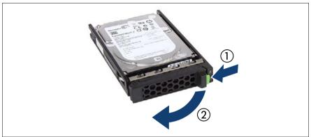
Figure 53: Opening the 2.5-inch HDD/SSD module locking lever
