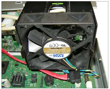
Figure 74: Cable routing for the first HDD fan module
