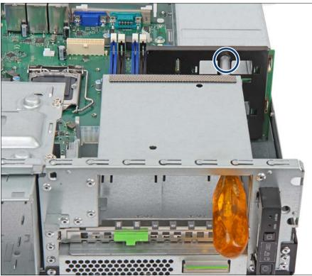
Figure 40: Replacing the power distribution board (B)
