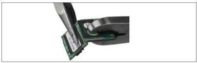
Figure 159: UFM breaking method
