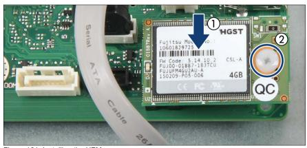
Figure 161: Installing the UFM
