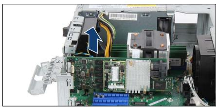
Figure 95: Removing an expansion card
