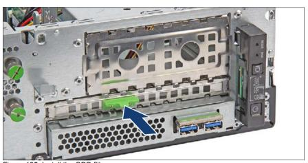
Figure 135: Install the ODD filler cover
