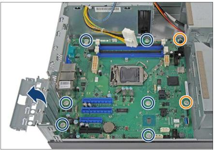
Figure 176: Screws system board
