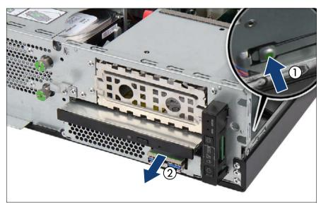
Figure 105: Removing the FBU holder
