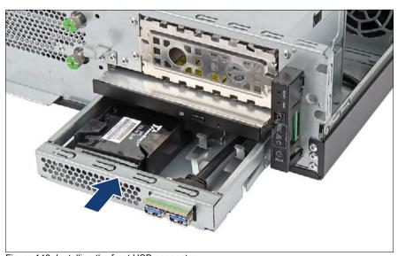
Figure 148: Installing the front USB connector
