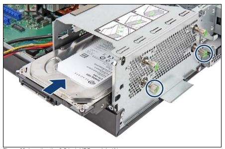
Figure 63: Inserting the 3.5-inch HDD module (A)
