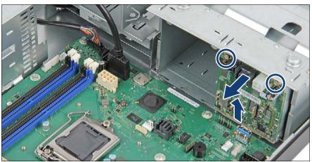
Figure 56: Removing the HDD backplane
