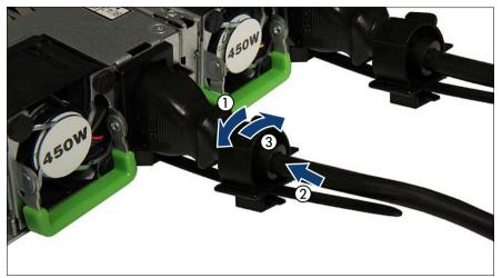
Figure 16: Example: Locking the cable clamp of a PSU
