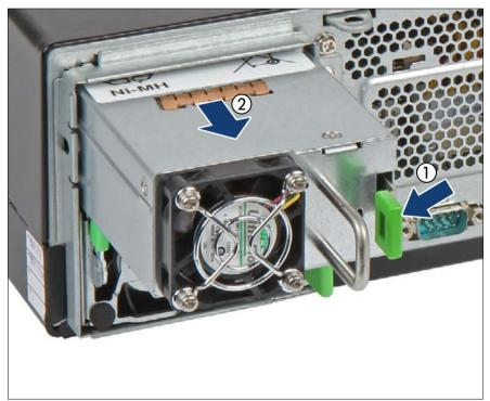
Figure 43: Removing a FJBU
