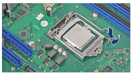
Figure 122: Latching the socket lever
