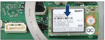
Figure 155: Installing the UFM
