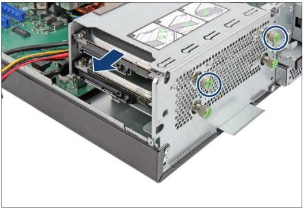
Figure 67: Removing the 3.5-inch HDD module
