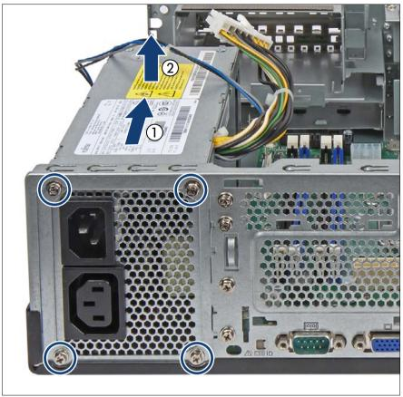
Figure 26: Removing the PSU
