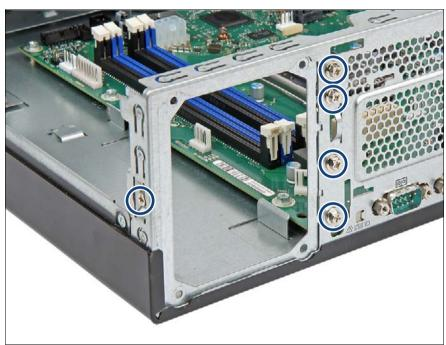
Figure 44: Removing the standard PSU frame (A)
