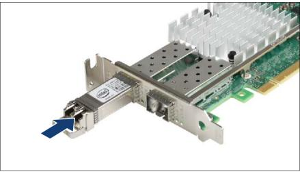
Figure 85: Inserting the SFP+ transceiver module
