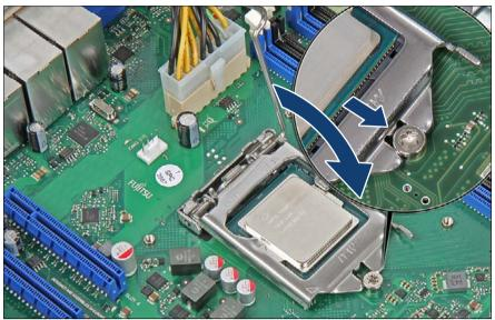
Figure 121: Closing the load plate (B)
