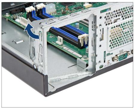
Figure 45: Removing the standard PSU frame (A)
