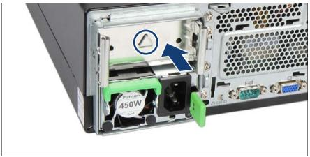
Figure 35: Installing a dummy cover
