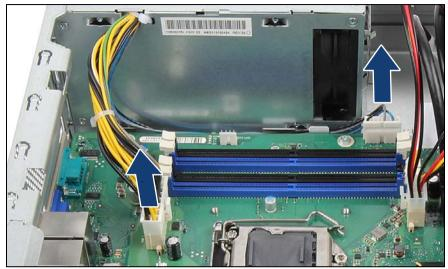
Figure 25: Disconnecting the power cables
