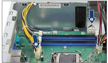
Figure 29: Connecting internal power cables
