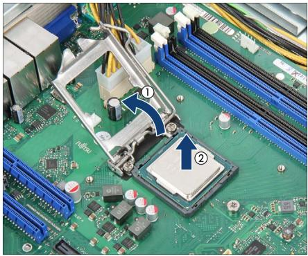
Figure 118: Removing the CPU
