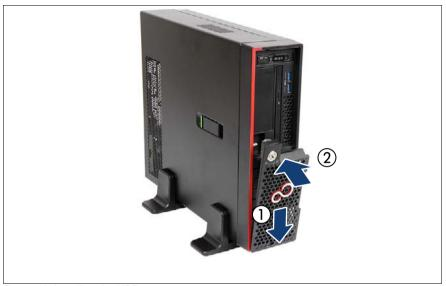
Figure 12: Installing the HDD cover
