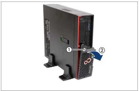
Figure 10: Removing the HDD cover
