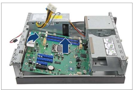
Figure 177: Removing the system board
