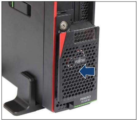
Figure 9: Placing the drive cover in front of the HDD cover
