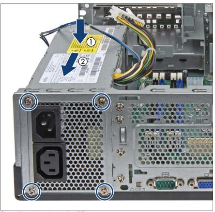
Figure 28: Installing the standard PSU
