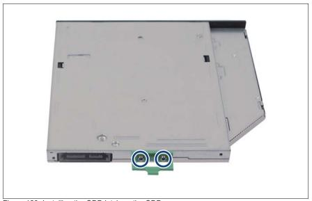
Figure 129: Installing the ODD latch on the ODD
