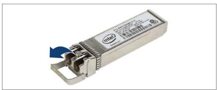
Figure 84: Unlatching the locking bail
