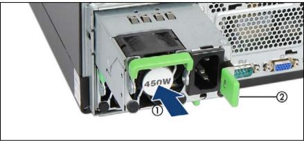
Figure 32: Installing a hot-plug PSU
