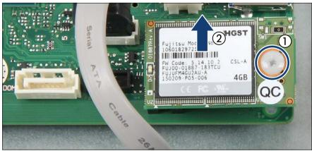
Figure 156: Removing the UFM
