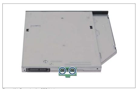
Figure 134: Removing the ODD latch
