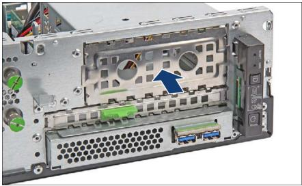
Figure 142: Inserting the drive filler cover
