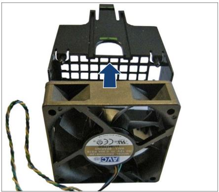
Figure 72: Example: Installing the fan into the holder (2.5-inch)
