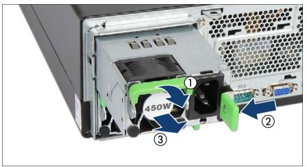
Figure 34: Removing a hot-plug PSU
