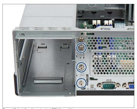
Figure 48: Installing the redundant PSU frame (A)
