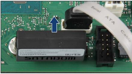
Figure 172: Removing the SATA DOM
