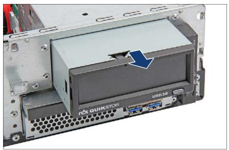
Figure 141: Removing the RDX drive (B)
