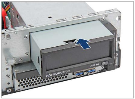
Figure 137: Installing the RDX drive (A)
