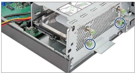
Figure 64: Inserting the 3.5-inch HDD module (B)
