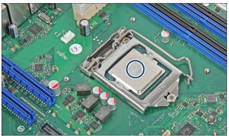
Figure 124: Applying thermal paste
