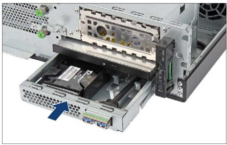
Figure 107: Installing the FBU (B)
