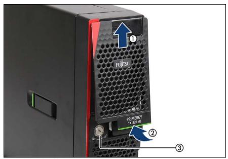
Figure 13: Installing drive cover
