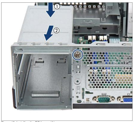
Figure 46: Installing the PSU cage (A)
