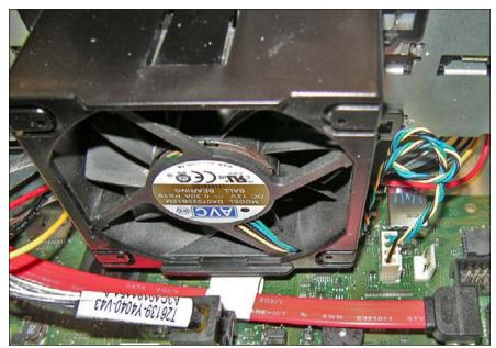
Figure 78: Cable routing for the HDD fan module
