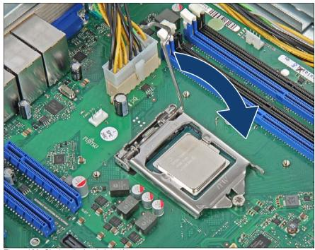
Figure 120: Closing the load plate (A)
