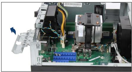
Figure 92: Opening the PCI slot bracket clamp
