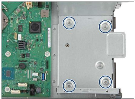
Figure 21: Recesses for the HDD cage (A)
