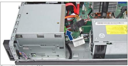
Figure 132: Unlocking the ODD
