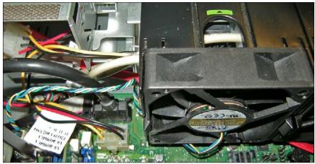
Figure 75: Cable routing for the second HDD fan module
