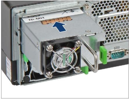
Figure 42: Installing a FJBU
