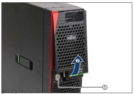
Figure 8: Removing the drive cover
