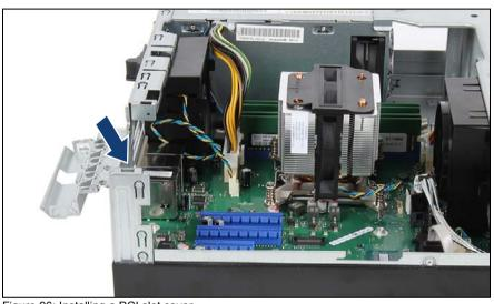
Figure 96: Installing a PCI slot cover
