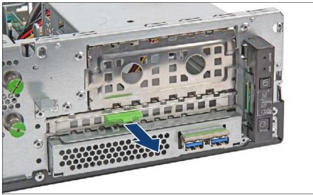
Figure 127: Removing the ODD filler cover
