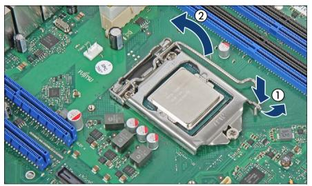
Figure 117: Unlatching the socket lever
