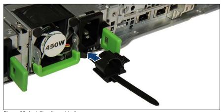
Figure 33: Installing the cable tie
