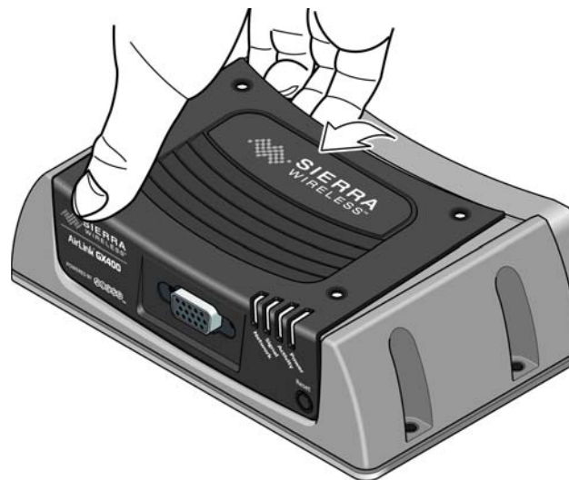
Figure 2-8: Tilting the cover (I/O X-Card installed)
