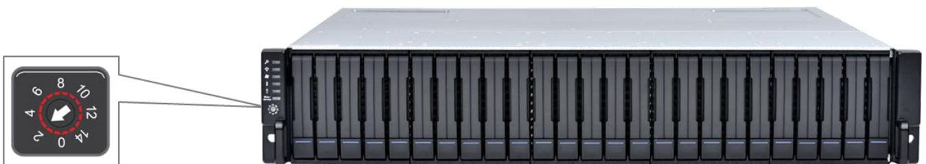
Figure 13: Expansion enclosure ID
