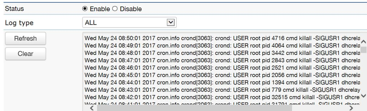
The screenshot shows the System Log interface. At the top, there is a "Status" section with radio buttons for "Enable" (selected) and "Disable". Below this is a "Log type" dropdown menu set to "ALL". On the left side, there are two buttons: "Refresh" and "Clear". The main area displays a list of log entries, each starting with a timestamp and followed by system information and a command. The entries are as follows:
