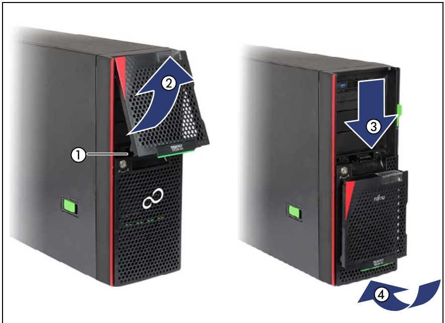
Figure 5: Removing the drive cover and placing it on the HDD cover
