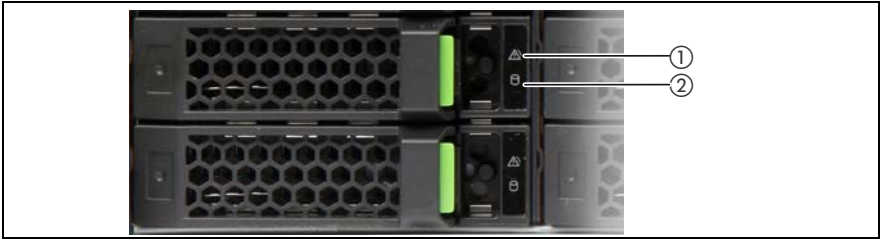
Figure 9: Indicators on the 3.5 inch HDD modules
