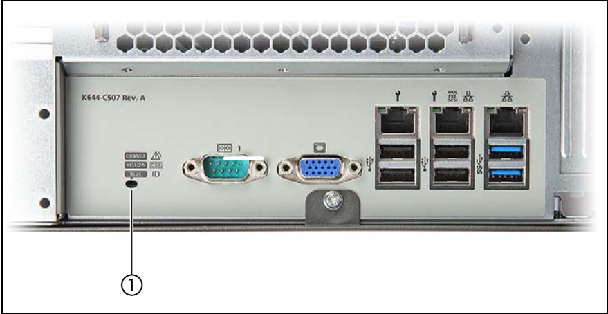
Figure 11: Indicators on the connector panel: CSS, Global Error and ID indicators
