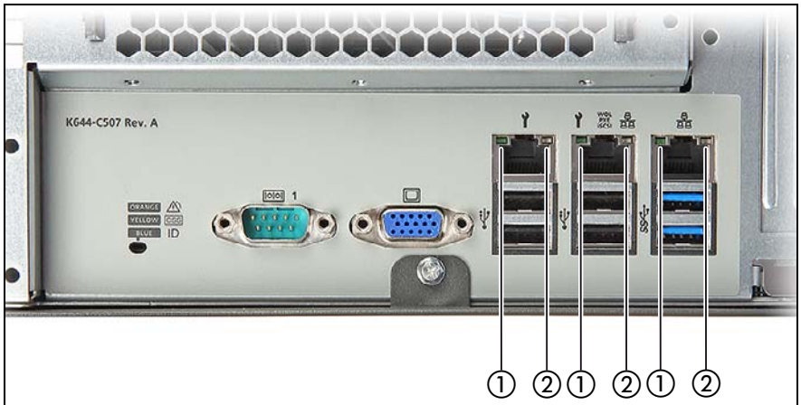
Figure 12: Indicators on the connector panel: LAN indicators
