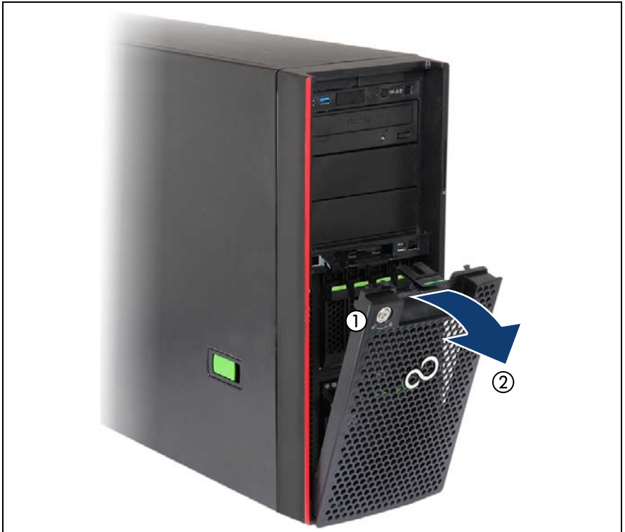
Figure 6: Removing the hard disk cover
