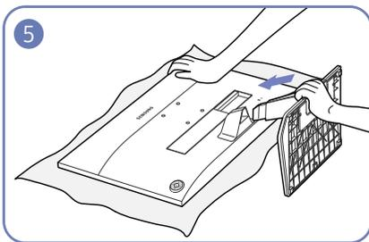
Insert the stand head into the connection hole in the direction, as shown in the figure.
