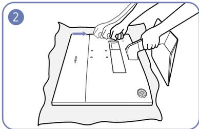
While holding the stand neck with one hand, pound the other fist down onto the top of the stand base in the direction of the arrow to detach the stand base.
