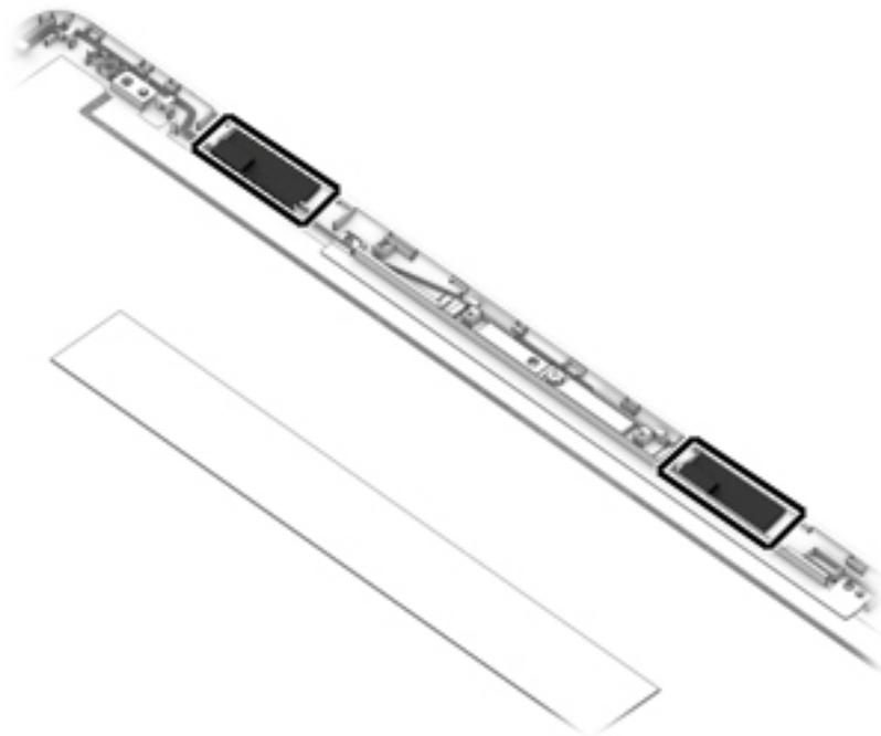
6. To remove the display/camera cable, remove the cable from the clips built into the side of the display enclosure (1), and then remove the cable from the display enclosure (2).
