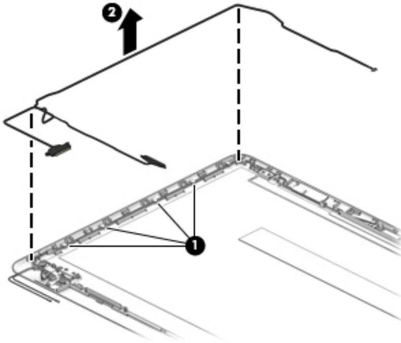
7. Use the following image to determine proper cable routing around the left hinge for the camera/display cable and the wireless antenna cables.
