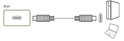
When a device outputs signals to the monitor using a USB Type-C cable, if the screen is not displayed normally, change the DP OUT output mode (switch the output mode between USB Type-C:MST and USB Type-C:SST).
