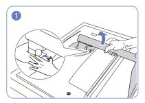
Place the product on a clean and flat floor as shown in Lift the stand nec the figure. Push the key upward and hold. Turn the stand from the display. neck of the display counterclockwise for 10°.
