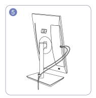
Arrange each of the two cables through either side of the COVER-STAND CABLE, as shown in the figure.
