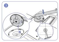
Place the stand neck on the display, as shown in the Turn the stand neck of the display clockwise for 90° figure. When you place the stand neck, ensure that the raised button on the display can be inserted into the groove of the stand neck.
