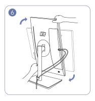
Rotate the machine to the horizontal position.
