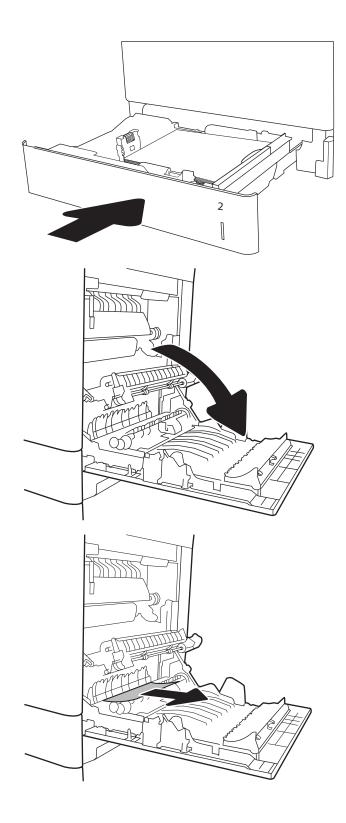
7. If paper is visible entering the bottom of the fuser, gently pull downward to remove it.
