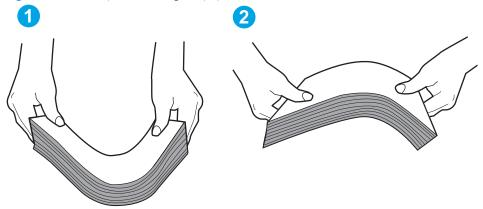
Figure 6-3 Technique for flexing the paper stack
