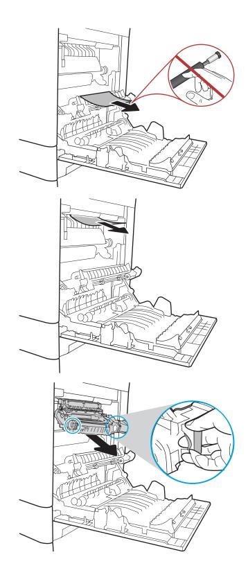
**13.** Open the jam-access door on the fuser. If paper is jammed inside the fuser, gently pull it straight up to remove it. If the paper tears, remove all paper fragments.
