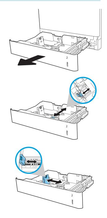
Load paper into the tray. Check the paper to verify the guides lightly touch the stack, but do not bend it. For information about how to orient the paper, see <u>Table 2-2 Tray 2 and the 550-sheet trays</u> paper orientation on page 27.
