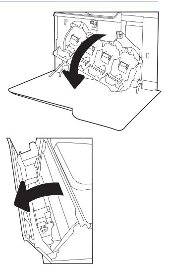
**3.** Grasp the top of the toner-collection unit and remove it from the printer.
