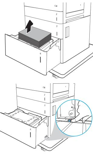
5. Lift the tray up and then pull it straight out to remove it.
