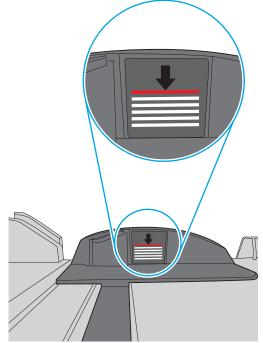
Figure 6-7 Tab for the paper stack
