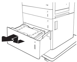
6. If jammed paper is in the feed area, pull it down to remove it. First pull the paper to the left to release it, and then pull it forward to remove it.
