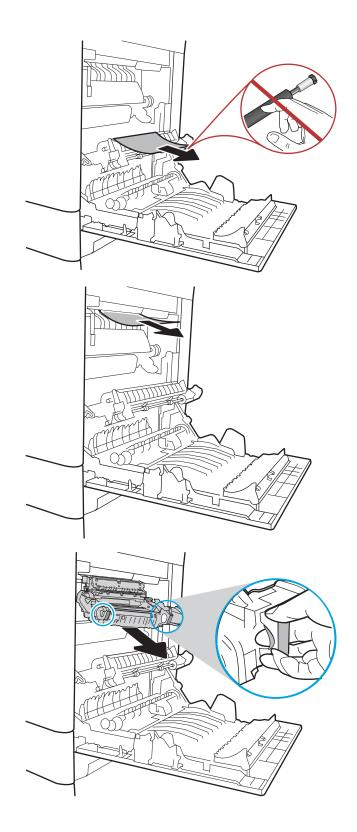
**10.** Open the jam-access door on the fuser. If paper is jammed inside the fuser, gently pull it straight up to remove it. If the paper tears, remove all paper fragments.
