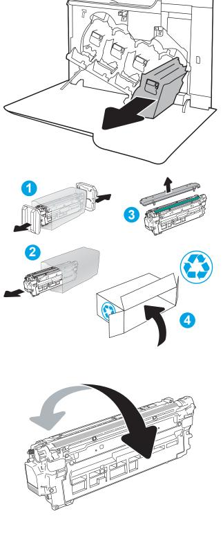
5. Support the toner cartridge underneath with one hand while holding the cartridge handle with the other. Align the toner cartridge with its slot on the shelf, and then insert the toner cartridge into the printer.
