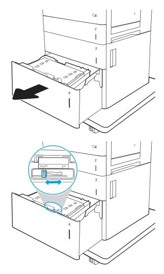
3. Rotate the paper-stop lever to the correct position for the paper being used.
