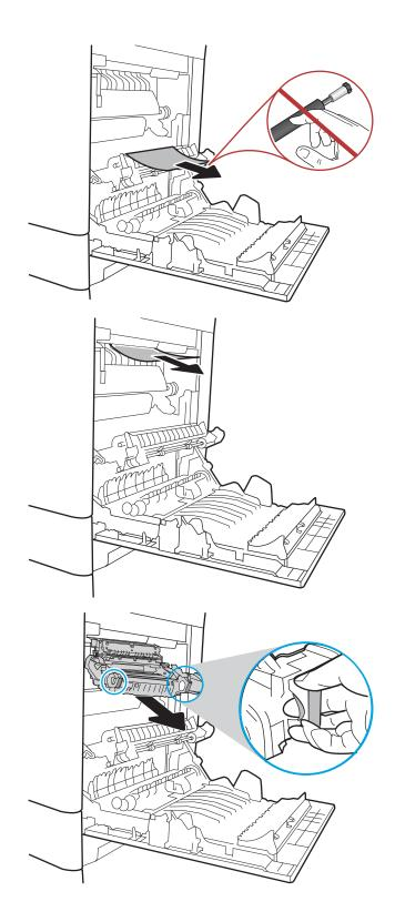
6. Open the jam-access door on the fuser. If paper is jammed inside the fuser, gently pull it straight up to remove it. If the paper tears, remove all paper fragments.
