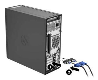
2. Connect the other ends of the monitor cables to the monitors.
