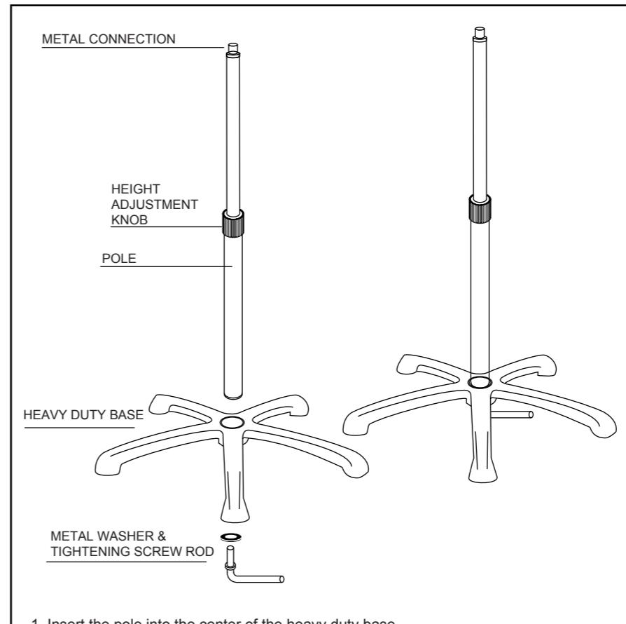
1. Insert the pole into the center of the heavy duty base.
