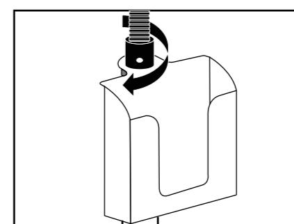
2. Place gooseneck over metal connection and turn clockwise to tighten.
