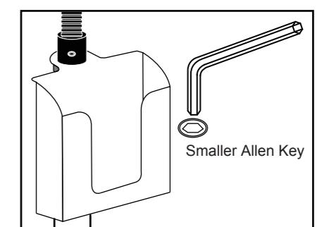
3. Use smaller Allen key to tighten the meter screw inside the gooseneck.
