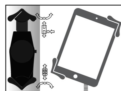
1. Press the button on the side of the holder center to slide out holder arm. Insert your tablet against the spring end, then slide the other arm back in, closing firmly.
