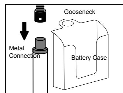
1. Place battery pack cradle over top of the pole's metal connection.
