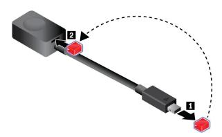
2. Connect one end of the Ethernet extension adapter to the mini Ethernet connector on your computer. Then connect the other end to an Ethernet cable.
