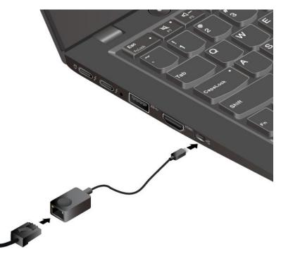
The Ethernet connector has two indicators that show the status of the network connection. When the green indicator is on, the computer is connected to a LAN. When the yellow indicator blinks, data is being transmitted.
