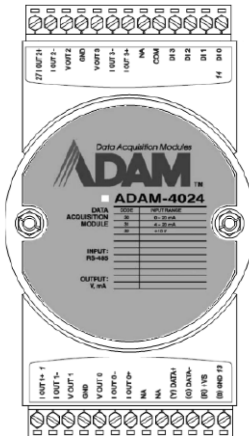
Figure 3.20 ADAM-4024 4-channel Analog Output Module
