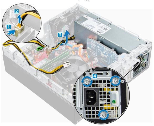
5 Press the blue release tab [1], slide the PSU and lift it away from the computer [2].
