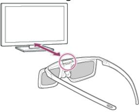
The Active 3D Glasses turn on and registration starts (the (1) (Power) button/indicator blinks green and yellow). When registration is finished, a message appears in the TV screen for 5 seconds, and the indicator lights up in green for 3 seconds.
