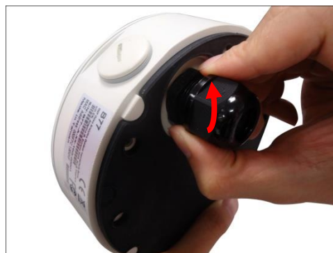
Attach to Camera Bottom Hole
