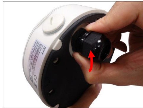
Attach to Camera Bottom Hole
