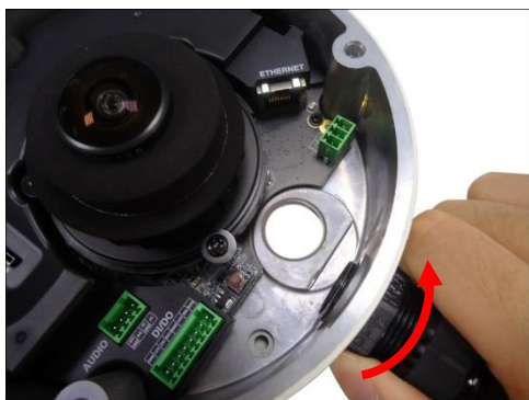
Attach to Camera Side Hole
