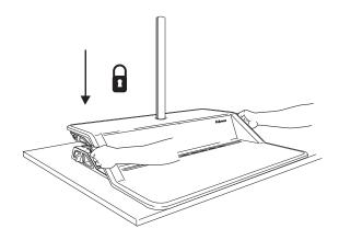
**Step 6**Install ring with the larger diameter downward.
