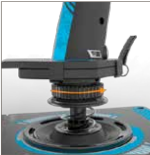
1. Turn Locking Bezel counterclockwise
