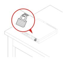
Locking the computer cover helps prevent unauthorized access to the inside of your computer. Your computer features a padlock loop so that the computer cover cannot be removed when a padlock is installed.
