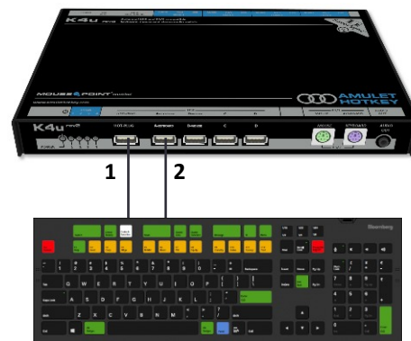
Model STB100: Bloomberg keyboard connected to USB hot-plug port (1) and USB keyboard socket (2) on the K4u+.
