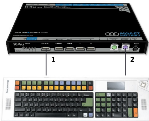
Models SEA100 and FRE100: Bloomberg keyboard connected to USB hot-plug port (1) and PS/2 keyboard socket (2) on the K4u+.
