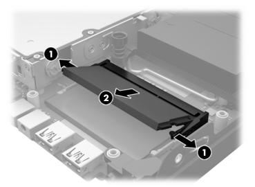
10. Slide the new memory module into the slot at approximately a 30° angle (1) then press the memory module down (2) so that the latches lock it in place.
