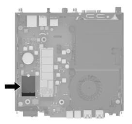
6. Disconnect both antenna cables from the WLAN module.
