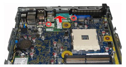
To install the expansion connector board, reverse the removal procedures.
