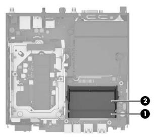
**9.** To remove a memory module, press outward on the two latches on each side of the memory module (1), and then pull the memory module (2) out of the slot.
