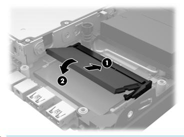
NOTE: A memory module can be installed in only one way. Match the notch on the module with the tab on the memory module slot.
