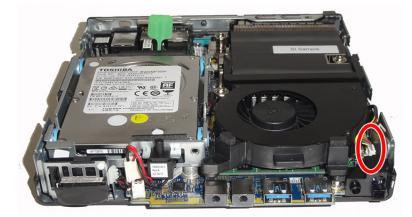
4. Lift the tab on the outer edge of the fan and rotate the fan upward, and then lift the fan out of the chassis.
