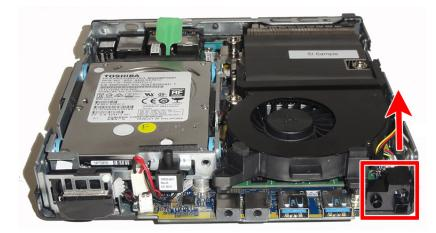
To install the power switch/light cover, reverse the removal procedure.
