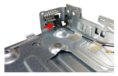
**16.** Remove the rear antenna from the inside of the computer by pressing the tab to disengage the transceiver and removing the transceiver (arrow in following image points to the tabs on the inside of the computer).
