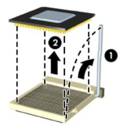
Reverse the removal procedure to install a new processor.
