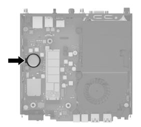
NOTE: You may need to use a small tool, such as tweezers or needle-nose pliers, to remove and replace the battery.
