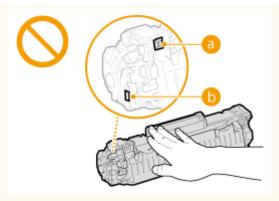
Do not scratch the drum surface ( ) or expose it to light.
