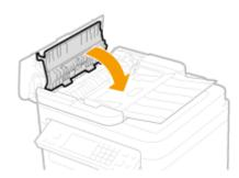
**3** Return the lever back in place, and close the feeder cover.
