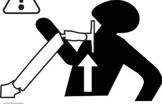
**EN** WARNING! Stored Energy Hazard: The arm mechanism is under tension and will move up rapidly, on its own, as soon as attached equipment is removed. For this reason, DO NOT remove equipment unless the arm has been moved to the highest position! Failure to follow this instruction may result in serious personal injury and/or equipment damage!
