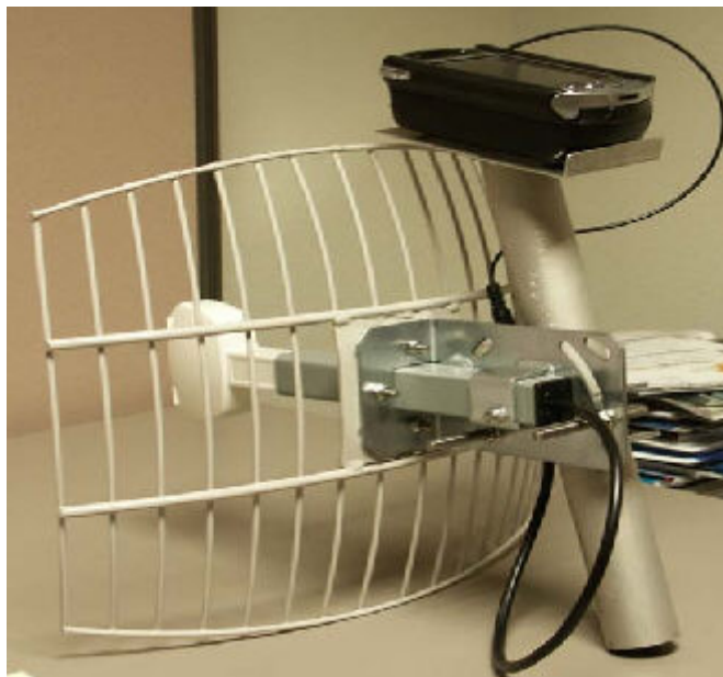
Tracking down noise source of RF jamming attack using the AirMagnet Handheld Analyzer on a Pocket PC
