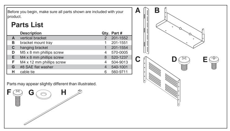
Attach hook bracket (not included) and hanging bracket (**C**) to screen with four M4 x 12 mm phillips screws (**F**) and #8 SAE flat washers (**G**).
