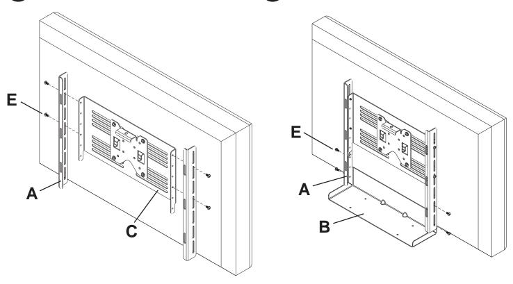
Attach VCR mount (not included) to bracket mount tray ( $\mathbf{B}$ ) with four M5 x 8 mm phillips screws ( $\mathbf{D}$ ). Use cable ties ( $\mathbf{H}$ ) for cord management once screen is attached to mount.
