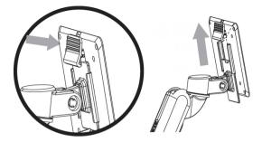
3. Attach the display to the Mount Bracket using the 4 Thumb Screws (3).
