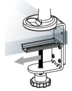
**Note:** The Desk Clamp can support a desk / table thickness from  $\frac{3}{4}$  - 4.3in (20 – 110mm). Depending on the thickness of your desk / table, the clamp can be adjusted smaller by removing the 4 screws and raising the bottom portion of the clamp as shown below.
