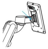
To increase / decrease swivel resistance, adjust the set screws located beneath the swivel points using a Phillips screwdriver, or on the base of the arm using the 3mm Allen Wrench (5).
